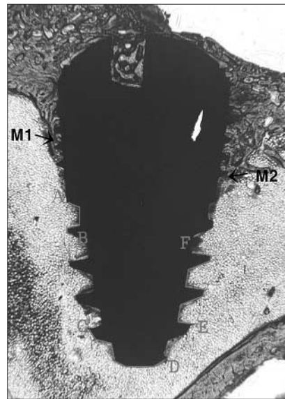
Fig. 1. Photomicrograph of the ground section (Villanueva bone stain; original magnification ×10). The length of the threads which were not attached to the bone(A to B, C to D and E to F) was measured first, and then it was subtracted from the whole length of the implant threads(M1-M2).
