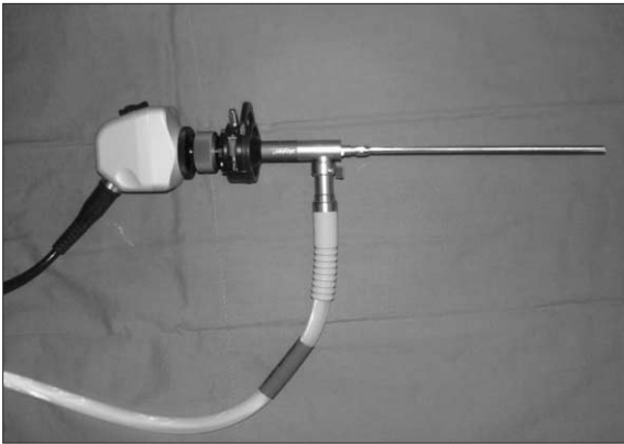
Fig. 3. Photograph of the Stryker endoscope assembled with three-chip camera head and fiber bundle.
