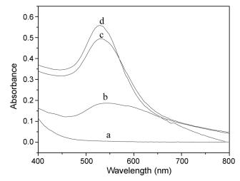
**Figure 1**. UV-Vis Spectra of (a) mixed solution containing HAuCl<sub>4</sub>, CTAB, and NaOH before UV irradiation and Au nanocrystals produced during the course of UV irradiation for (b) 3 h, (c) 6 h, (d) 9 h.
