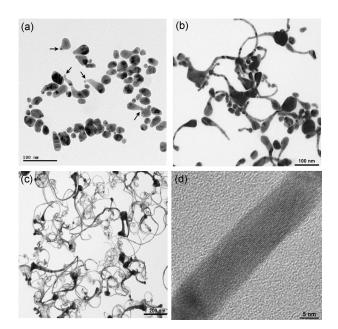
Figure 2. TEM images of the gradual evolution of Au nanowires during UV irradiation for (a) 3 h, (b) 6 h, (c) 9 h. Tadpole-shaped Au nanoparticles are indicated with arrows in (a). (d) High-resolution TEM image of a gold nanowire.
