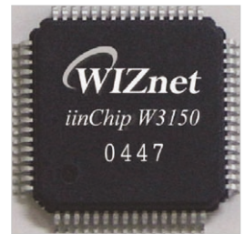
[Hardwired TCP/IP Chip_W3150]
