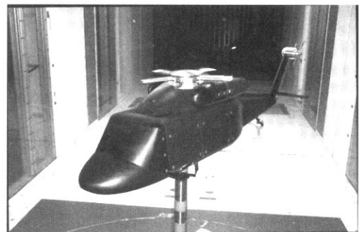
Fig. 2. Fuselage model (1:8) in ADD-LSWT
