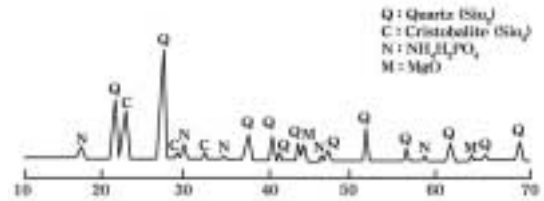
〈Fig. 1〉 The X-ray diffraction patterns of Rema®Exakt investment(Dentaurum Co., Germany) used in this study.
