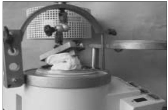
Fig. 4. After selecting 4mm foil for Medium type, embed model with the 1st.
