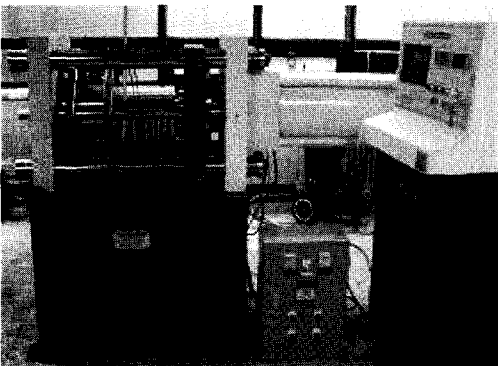
Fig.13 The photo of hot metal extru-bending Machine
