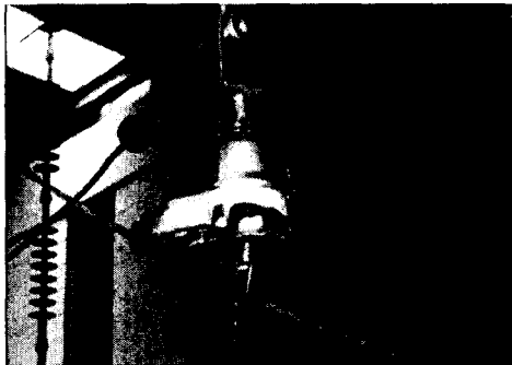
(c) 5분경과(파손상태) (5 minutes elapsed, breakage disc)
