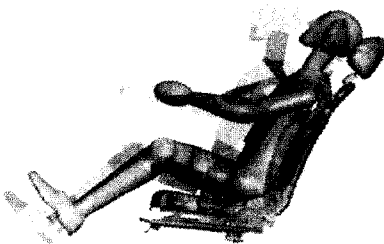
Fig. 14 Deformed shape(FMVSS 301 test)
