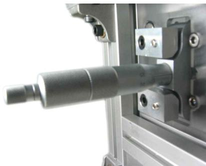
Fig. 5 Depth  $\mu$ -meter for clearance control
