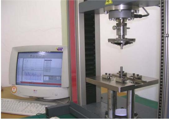
Fig. 3 Experimental setup for fracture strength test by UTM
