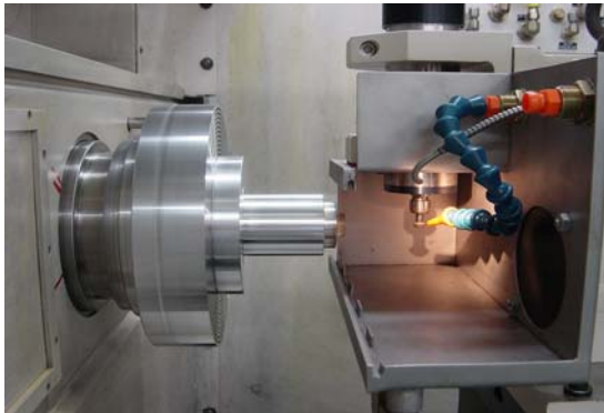
Fig. 4 Grinding for ultra-precision aspheric surface
