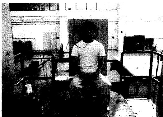
Fig. 2 Picture of the head vibration measurement using the 12-axis bite-bar
