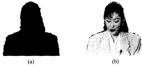
Fig. 13 Object extraction with second mask (Akiyo) (a) Moving object mask, (b) Segmentation result
