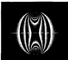
Fig. 10 Isochromatic fringe phase map obtained from Table 1 and Eq. (4) for 4-step phase measuring method
