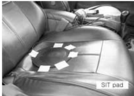
Fig. 2 Triaxial SAE pad sensor secured on the seat
