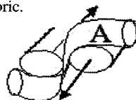
Figure 4. Deformation of the yarn in the twill weave.
