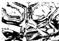
Fig. 3. Photomicrograph of serpentinite showing the points of analyses along the scanning line from olivine (O1-O3) to serpentine (S1-S7).
