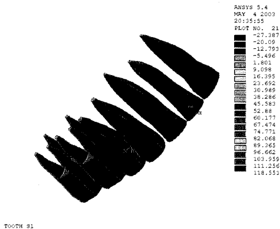
Fig 6. .019 x .025 SS 2° maximum principal stress.
