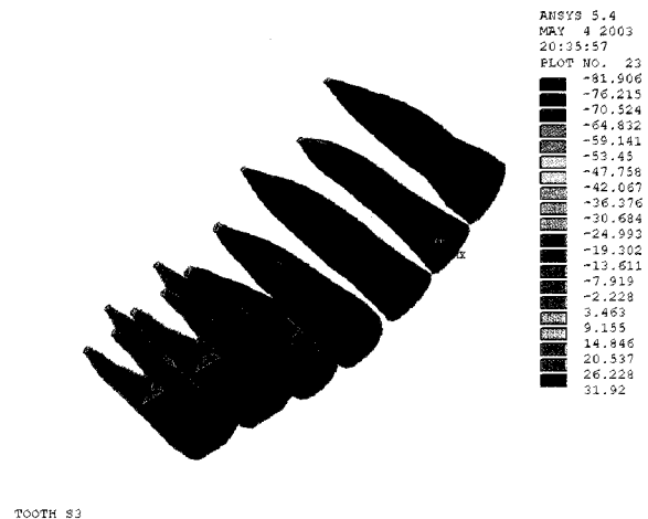
Fig 7. .019 x .025 SS 2° minimum principal stress.
