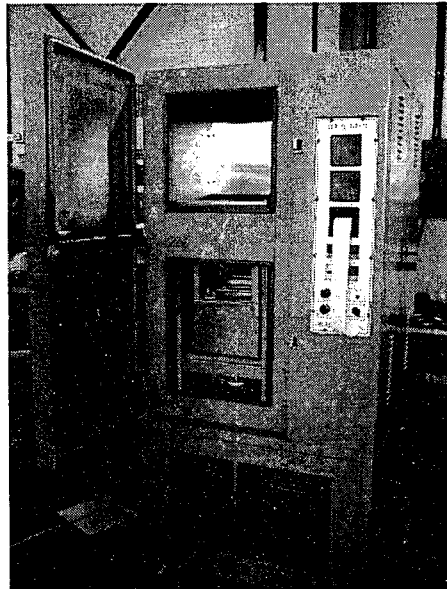
Fig. 5 Newly manufactured thermal impact experimental apparatus
