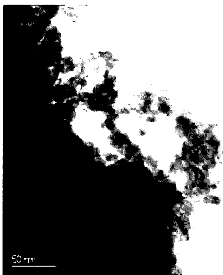
Fig. 1. TEM image of CuO particles. Before dispersed in liquid, particles are strongly aggregated.
