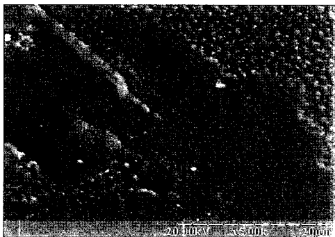
Fig. 2 The surface of polyimide after elimination surface debris using O 2 plasma system (HITACHI DRY MAX:150W).
