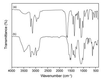
Figure 4. IR spectra of (a) cis-[Cr([14]-decane)(ox)]ClO<sub>4</sub>·(1/2)H<sub>2</sub>O and (b) cis-[Cr([14]-decane) (acac)] (ClO<sub>4</sub>)<sub>2</sub>·(1/2)H<sub>2</sub>O.
