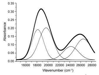
**Figure 3**. The electronic absorption spectrum of  $2.0 \times 10^{-3}$  M *cis*-[Cr([14]-decane)(ox)]<sup>+</sup> in DMF solution at 298 K.
