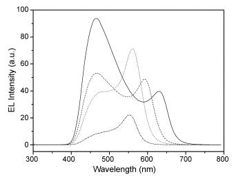
Figure 5. EL spectra of blue device,  $Al(200 \text{ nm})/2\text{-TNATA}(60 \text{ nm})/\text{NPB}(15 \text{ nm})/\text{DPVBi}(30 \text{ nm})/\text{Alq}_3(30 \text{ nm})/\text{LiF}(1 \text{ nm})/\text{Al}(20 \text{ nm})$ . Detection angle: (----):  $30^{\circ}$ , (----):  $30^{\circ}$ , (----):  $60^{\circ}$ , (----):  $90^{\circ}$ .
