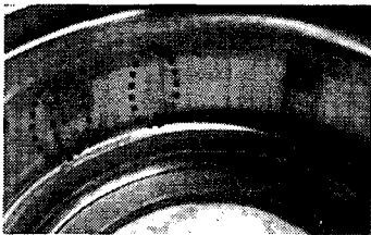
Fig. 11 Damage shape of an outer race the reverse-locking clutches after overload applied at 9,793 kgf-cm
