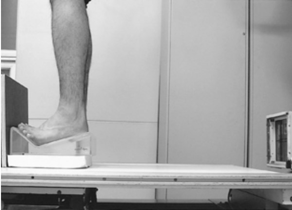
Figure 1. Photograph of the foot device used for taking radiographs of standing sesamoid tangential view.
