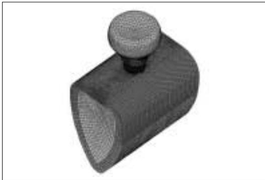
**Fig. 3.** Three-dimensional finite element model of full body.
