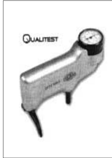
Fig. 12. Barcol hardness tester
