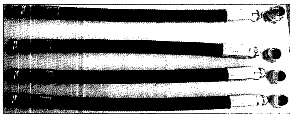
Fig. 6 Hoses for burst test
