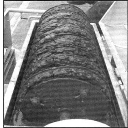
Fig. 6. Biofilms attached onto reticular rotating carrier of RABC reactor.
