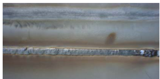
(e) 용접 전압 400V, 전류 400mA (e) Welding voltage : 400V, Welding current : 400mA
