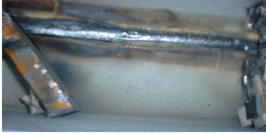
(f) 용접 전압 600V, 전류 400mA (f) Welding voltage : 600V, Welding current : 400mA
