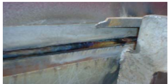
(c) 용접 전압 600V, 전류 200mA (c) Welding voltage : 600V, Welding current : 200mA
