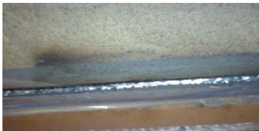
(a) 용접 전압 200V, 전류 200mA (a) Welding voltage : 200V, Welding current : 200mA
