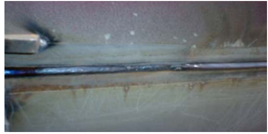
(b) 용접 전압 400V, 전류 200mA (b) Welding voltage : 400V, Welding current : 200mA
