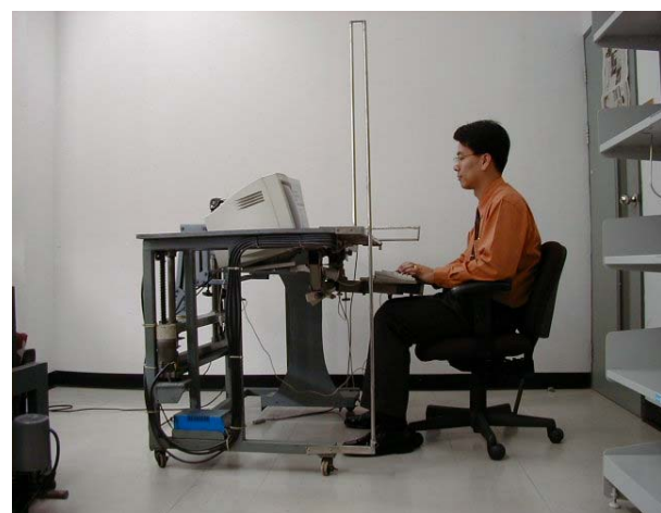
Figure 1. The subject's body posture when the workstation is adjusted according to the recommended settings
