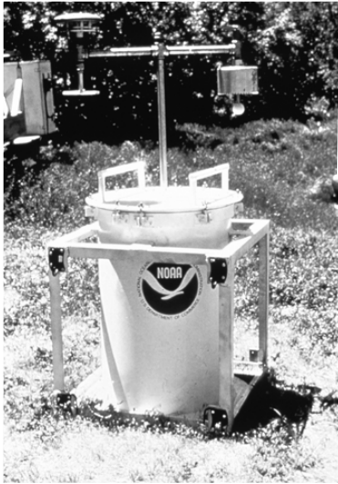
Fig. 1. TOTO outfitted with a variety of weather instruments – anemometers, pressure sensors and humidity sensors. Form NOAA (2004).
