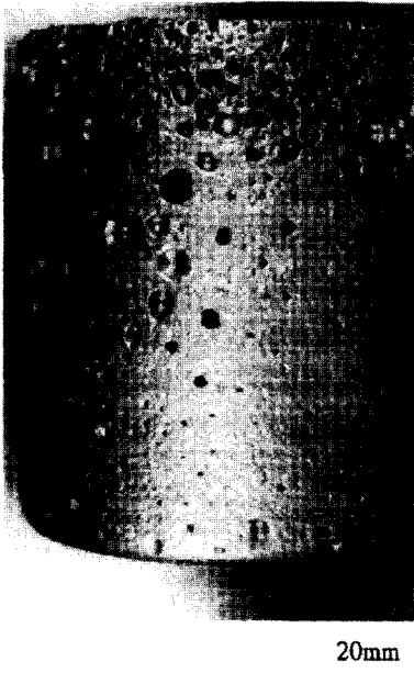
Fig. 11. Appearance of Ti-6Al-4V ingot melted in CaO crucible.
