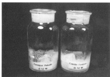
Photo 1. Wood block attacked by wood-rotting fungi.
