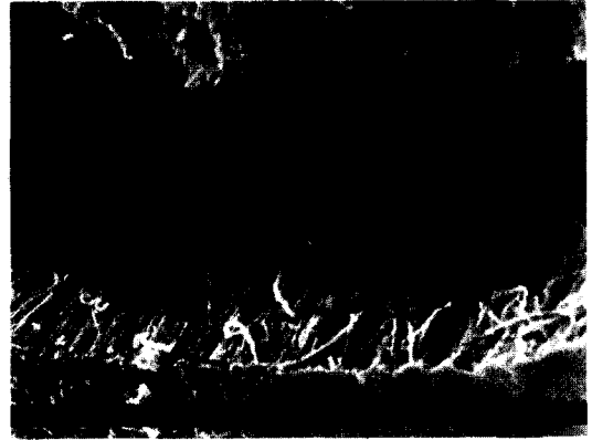
Fig. 2. SEM images of about 40 \mu\text{m} ( \downarrow )-thickness CdSe film: Cross-sectional SEM picture of CdSe film on epoxy.
