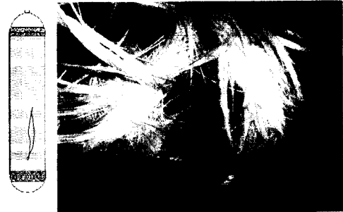
Fig. 8. Longitudinal failure mode of the tested cylinder
