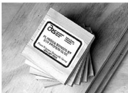
Figure 3. Plywood bonded by soy protein adhesives.
