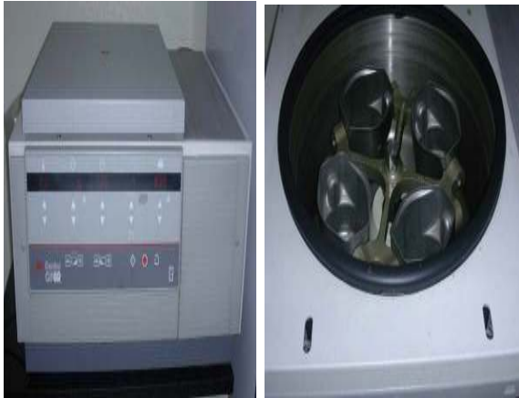
Fig. 5. IEC central GP8R centrifuge (IEC, Needham Heights, MA, USA) (left; outside view, right; inside view).
