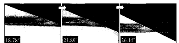
Fig. 10 Nozzle flow deflection as nozzle installation angle(Degree), Schlieren image
