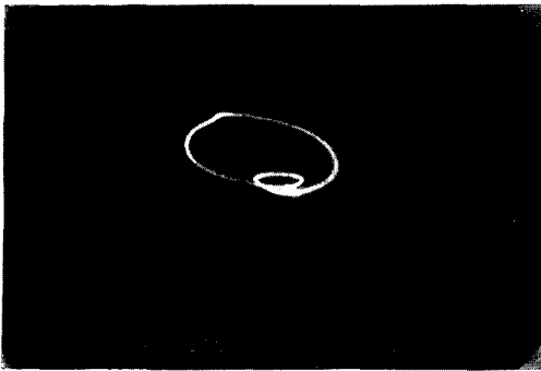
Fig. 6 Subharmonic motion and superharmonic motion at transverse 4th and torsion 2nd mode(788 Hz)
