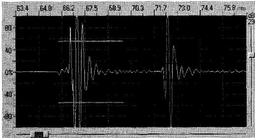
Fig. 6 The signal of debonding interface
