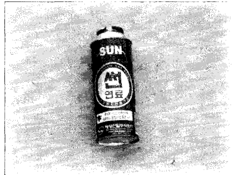
Fig. 6 Butane can before explosion(w : 134 g)
