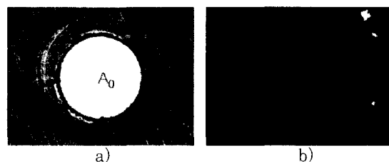
Fig. 3 Wear of contact tip: a) area of exit hole before welding, b) area of worn-out hole after 't' hour welding
