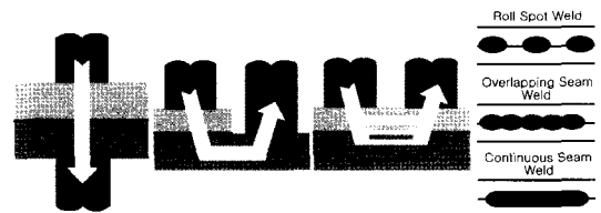
Opposed Welding Step Welding Series Welding Seam Welding
