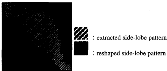
Fig. 3. Extracted side-lobe patterns and reshaping with EXTENTS function.
