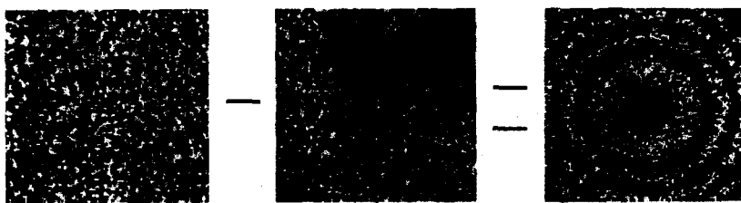
(a) Before deformation (b) After deformation (c) Fringe pattern Fig. 5. Fringe pattern obtained from the speckles before and after deformation
