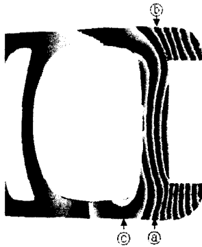
Fig. 8. Fringe pattern obtained from the initial sample before the durability test
