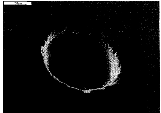
Fig. 18 Machined result with force feedback USM(tool= \phi 100 \mu )
