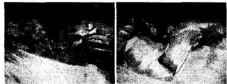
Fig. 7 Fractography of BMC specimen.
